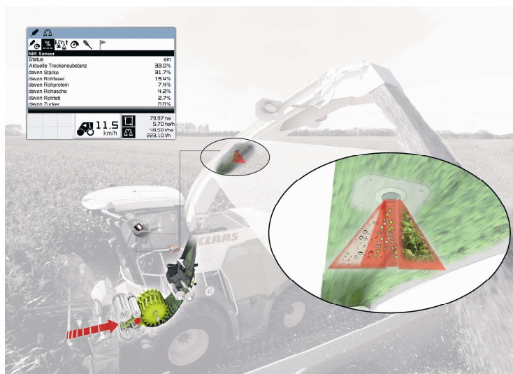
Figure 4 Online measuring of substrate qualities at harvest of Claas Inc [5]
