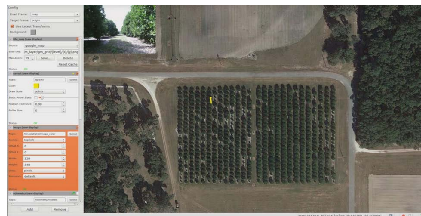
Figure 4. Developed program that visualizes the Google map, the GPS locations (the yellow line) and the live video stream (top-left corner of the map) from the Kinect.
