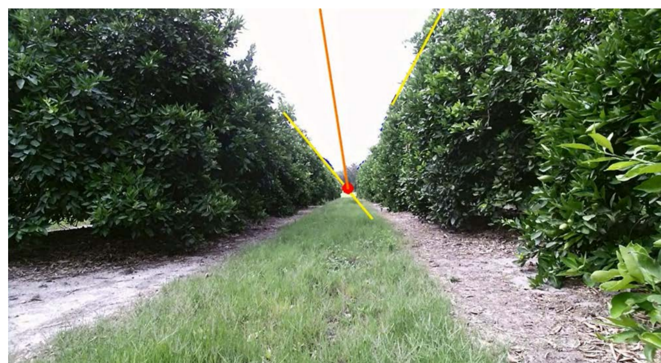
Figure 3. Machine vision for real-time central line (orange solid line) detection and robot's relative positions and orientations determination.
