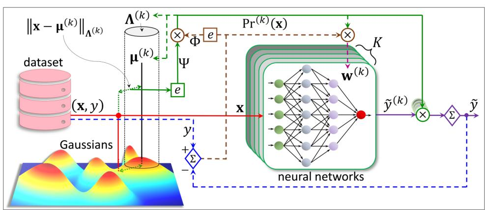
Fig 5: Schematic of proposed model, showing dataset, mixture of gaussians and deep neural networks.
