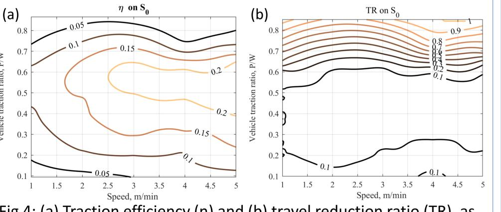
Fig 4: (a) Traction efficiency ( $\eta$ ) and (b) travel reduction ratio (TR), as
