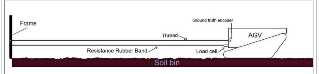
Fig 3: A conceptual drawing of drawbar pull test experimental setup.
