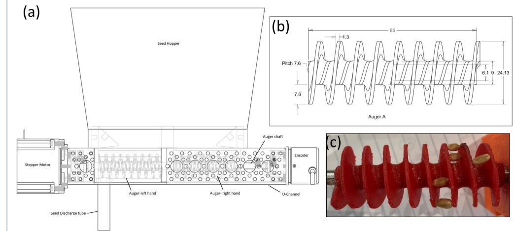
Fig 7: (a) Schematic of auger type feed metering unit, (b) designed auger (Dim. in mm) as per ASABE standard , (c) observed seed blockage on small pitch auger.
